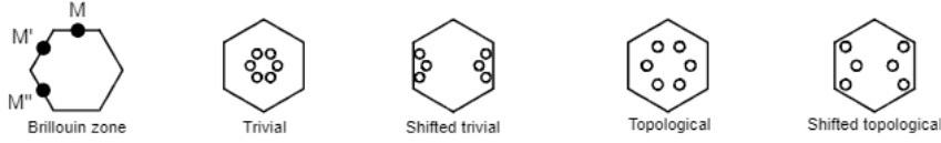
Figure C.1: Positions of M , M' , and M'' within the Brillouin zone, and schematics of the (shifted) shrunken-ring and expanded-ring unit cells introduced by Wu and Hu [1].
